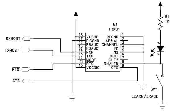
In some addressed mode applications the learn/erase components may not be required and the LRN/LED pin could be connected to the host micro controller which would be programmed to handle the functions of this pin.
